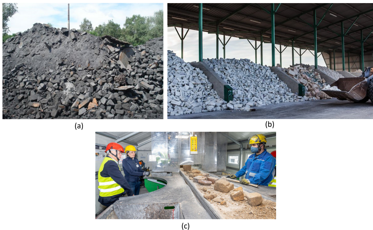
Figure 2 - (a) Spent MgO-C from steel furnace breakout [15]; b) Outdoor storage of spent refractories received at the recycling plant before treatments [16]; c) Manual sorting [17].
